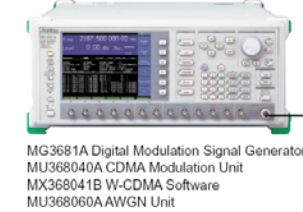
Signal generator for wanted signal and AWGN
